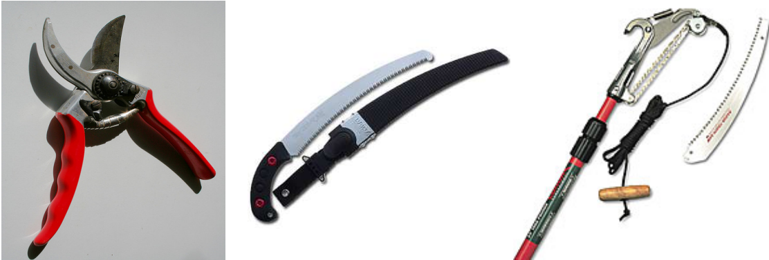
Figure 14: Three types of pruning tools. (L to R) 1) Bypass Hand Pruners, 2) Hand Saw, 3) Pole Saw or Pruner.
